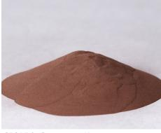
**C18150 Copper Alloy** Produced with 6K Additive UniMelt microwave plasma technology.
