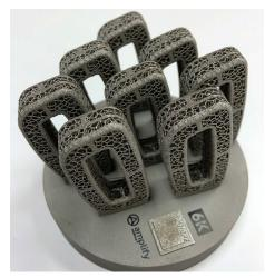
**Ti6Al4V Printed Spinal Cage** Spinal cages designed at Amplify Additive and printed on a Trumpf TruPrint 1000 LPBF system with 6K's Ti6Al4V powder.
