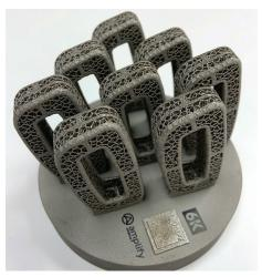
Ti6Al4V Printed Spinal Cage Spinal cages designed at Amplify Additive and printed on a Trumpf TruPrint 1000 LPBF system with 6K Additive's Ti6Al4V powder.
