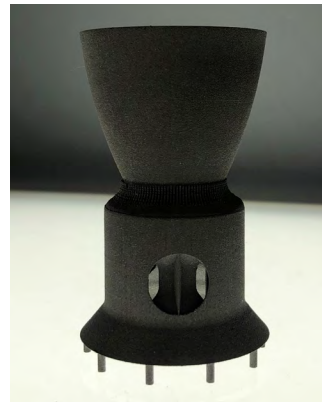
Non-eroding throat insert for a solid rocket motor nozzle. Printed by Quadrus using 6K Additive tungsten rhenium powder
