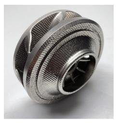
Ni625 Printed Impeller Industrial impeller printed using 6K Additive plasma spheriodized powder at Sintavia on an EOS M290 L-PBF system.
