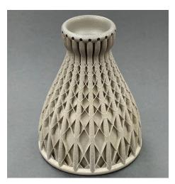
**Ni718 Printed Rocket Nozzle**Printed using 6K Additive plasma spheroidized powders at Castheon on a Concept
